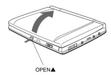
3 Put your finger on the pit DISC OPEN▲ on the left side of this unit and open the disc cover.
